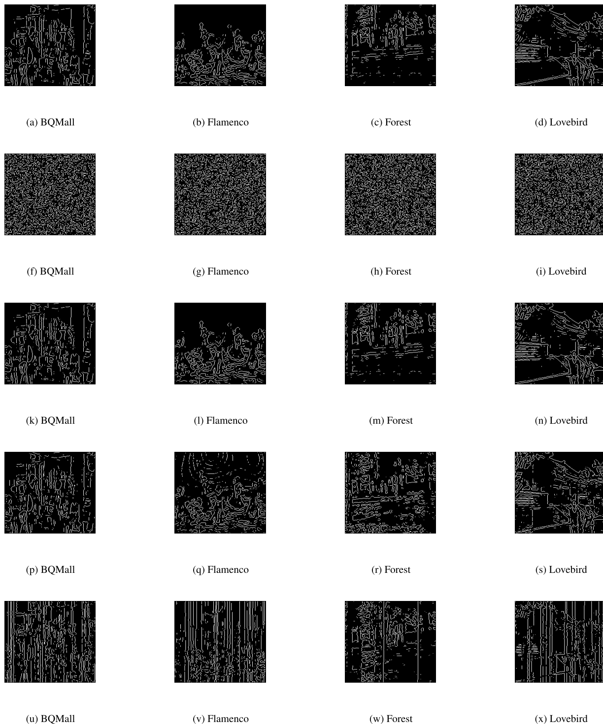
FIGURE 9. Edge detection outcomes for: (a: e) original video frame edges; (f: j) encrypted video frame edges; (k: o) decrypted video frame edges under low turbulence strength; (p: t) decrypted video frame edges under moderate turbulence strength; and (u:y) decrypted video frame edges under strong turbulence strength.
