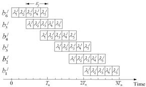
Fig. 1: The concept of overlapping among the bits of *class-j* users, showing the effect of the overlapping coefficient  $\mathcal{E}_{i}$  on their transmission rate.
