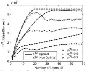
Fig. 9: The optimal throughput versus the total number of users for the two-class system.
