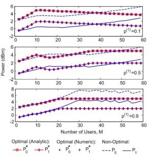
Fig. 8: The transmission power versus the number of users for a two-class system.
