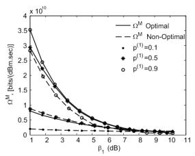
Fig. 5: The throughput versus QoS of *class-1* for different multimedia distributions.
