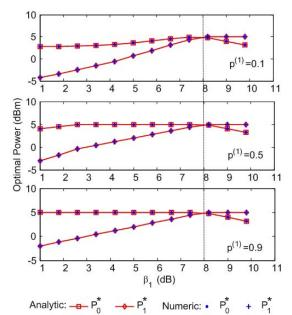
Fig. 4: The power consumption of *class-0* and *class-1* for different multimedia distributions.
