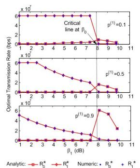
Fig. 3: The transmission rates versus QoS of *class-1* users for different multimedia distribution.
