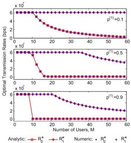
Fig. 6: The optimal transmission rates versus the number of users for a twoclass system.
