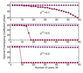
Analytic:  $\bullet \varepsilon_0^* \to \varepsilon_1^*$  Numeric:  $\bullet \varepsilon_0^* + \varepsilon_1^*$ Fig. 7: The optimal overlapping coefficient versus the number of users for a two-class system.
