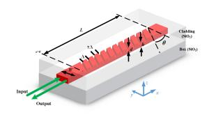
Fig. 1: Perspective view of proposed polarization rotator design.
