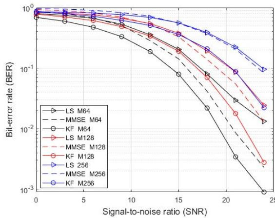
Figure 3. Comparison of BER performance for KF, LS, and MMSE.
