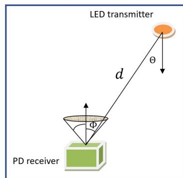
Figure 1. Geometry for a LOS propagation model.
