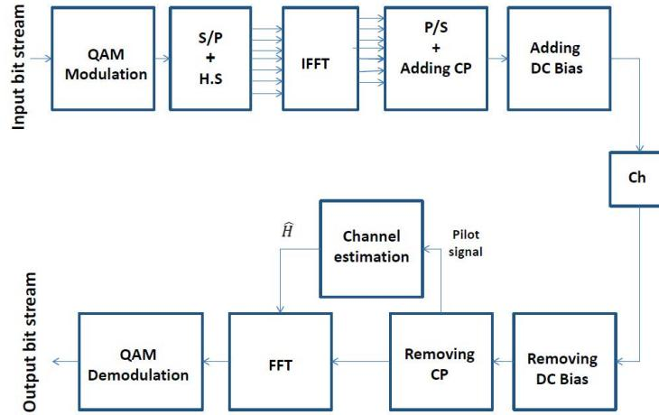
Figure 2. Block diagram of DCO-OFDM system.
