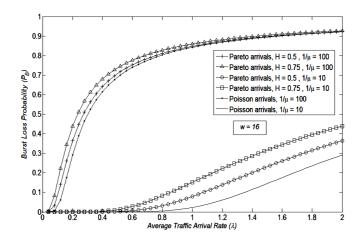
Fig. 2. Burst loss probability versus the average traffic arrival rate for FWC case for Poisson and Pareto arrivals at different values for the Hurst parameter and burst length.
