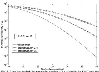
Fig. 3. Burst loss probability versus the number of wavelengths for FWC case for Poisson and Pareto arrivals at different values for the Hurst parameter.
