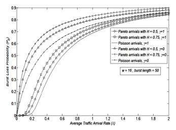
Fig. 1. Burst loss probability versus the average traffic arrival rate for NWC and FWC cases for Poisson and Pareto arrivals at different values for the Hurst parameter.
