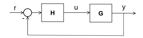
When open loop transfer func G changes by  $\Delta G$ , closed loop transfer func T changes by  $\Delta T$
