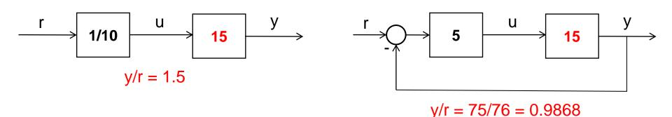
Closed loop less sensitive to change in plant gain
