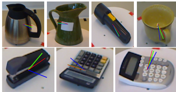
Figure 1. Ground truth and estimated poses overlaid for sample images. The red line signifies the ground-truth pose, green represents the estimated pose using visual + depth and blue is the estimated pose using visual local features only. 1
